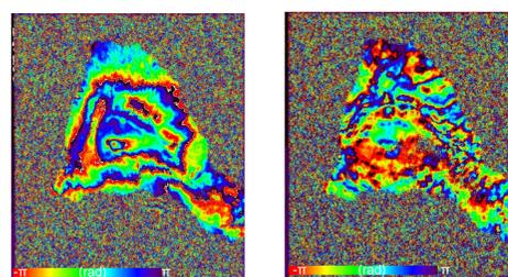
An example of the phase due to the low frequencies of the interferograms 20170923\_20170929 and 20180202\_20180208, after removing the phase correlated with topography from the respective interferograms using Fourier transforms.
