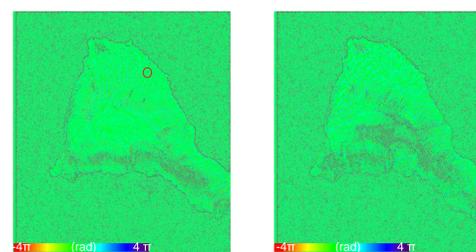
The phase of the residuals after of filtering the low frequency signals is shown in the figure. By preliminary qualitative analysis, it was observed that most of the deformations or movements existing in the given area was retained in the image
