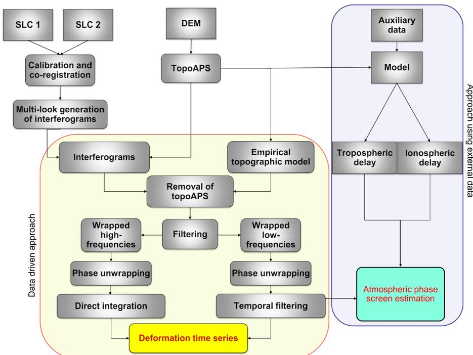
$$\Delta\varphi_{int} = \Delta\varphi_{deformation} + \Delta\varphi_{atmosphere} + \Delta\varphi_{noise} + \Delta\varphi_{topography} + 2k\pi$$
