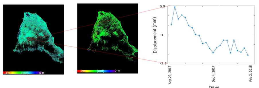
The figure above shows the accumulated deformation using the filtering and the standard PSIG chain. It shows a significant improvement in the spatial coverage of PSs and reduction in phase unwrapping errors. Also an example of the time series of a stable point is shown in the figure.
