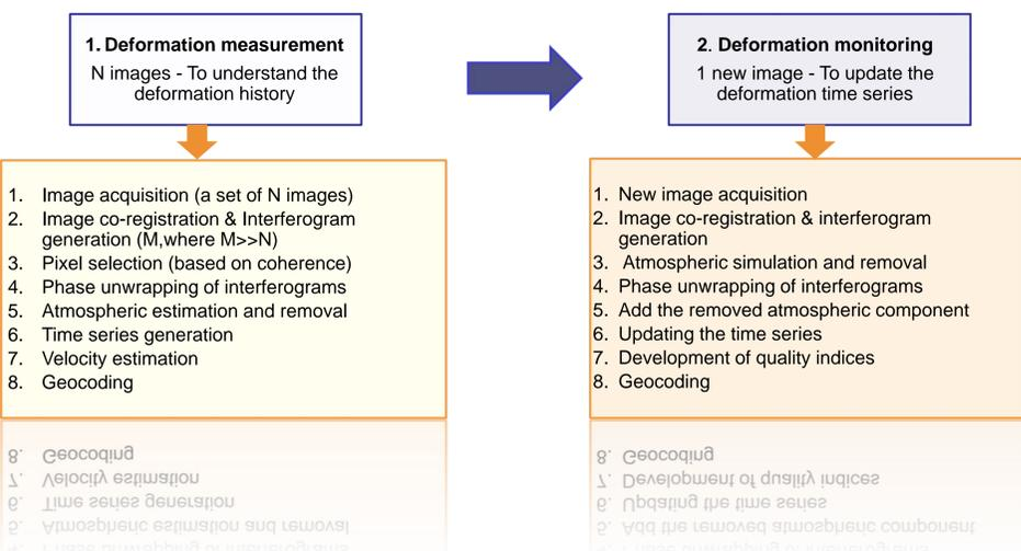
The main objective of the PSI chain was to extend interferometric processing to wider areas using a unique, redundant and connected network of points and any type of interferometric SAR data. The generated maps consist in a set of selected points (Persistent/Dispersed Scatterer (PS/DS)) containing the information of the estimated annual velocity and the accumulated deformation at each image acquisition time.
