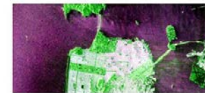
Fig. 1.8. Radarim-2 polarimetric: RGB image view San Francisco (USA) when the colour code is: I_{hh} , I_{hv} , I_{vh} and I_{vv} , green. Filtered image with the LLMMSE speckle filter.
