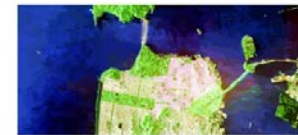
Fig. 1.9. Radarim-2 polarimetric: RGB image view San Francisco (USA) when the colour code is: I_{hh} , I_{hv} , I_{vh} and I_{vv} , green. Filtered image with the SPT speckle filter.
