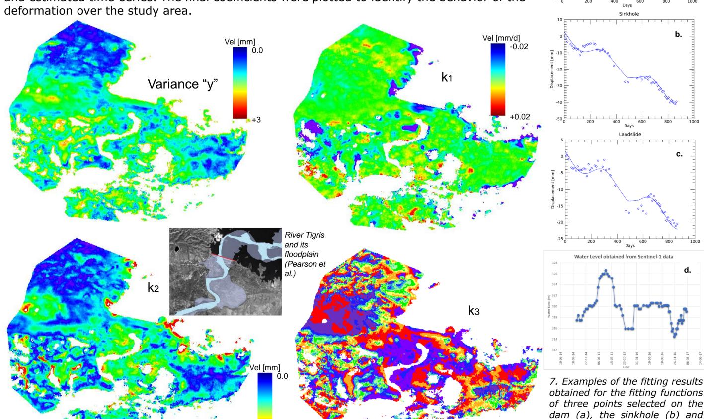
6. Results of the fitting coefficients obtained from the variance minimization. The variance 'y' was used as a degree of confidence to mask the other parameter maps. k1 represents the entity of linear component of vertical displacements; k2 is the amplitude of the oscillation, giving information on the influence of the seasonal behavior; k3 is the initial phase of the oscillation, showing the spatial propagation of the oscillations and its timely delay.
