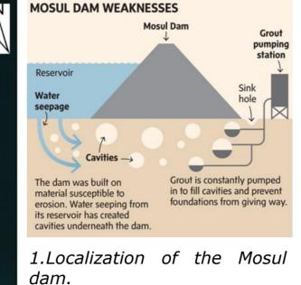
2. Formation of underground cavities, causing the dam instabilities. Grouting injections were adopted as consolidation.
