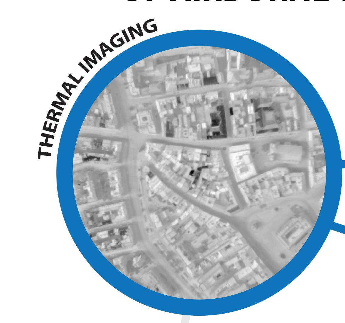
Thermal camera used for imaging (FLIR Tau2) was calibrated by the manufacturer. However, laboratory testing measurements were performed at our department. After the flight, one of the most obvious errors was vignetting. Due to the sensor structure, the angle of imaging results in much higher error than with other convention remote sensing methods.
