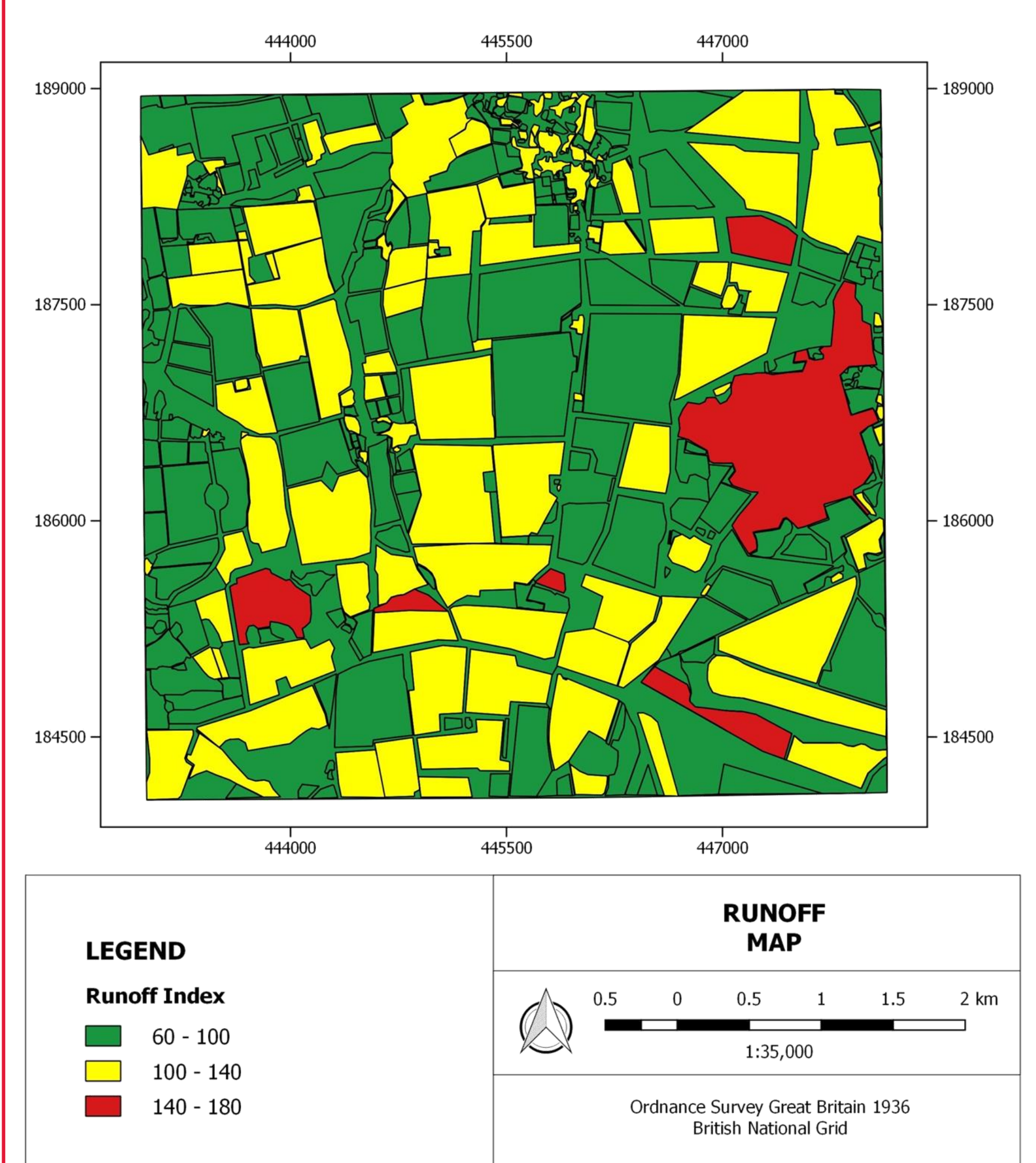
Fig. 9: Runoff Hazard index map (June 2016). Green=low hazard; Yellow=Moderate hazard; Red=High hazard.
