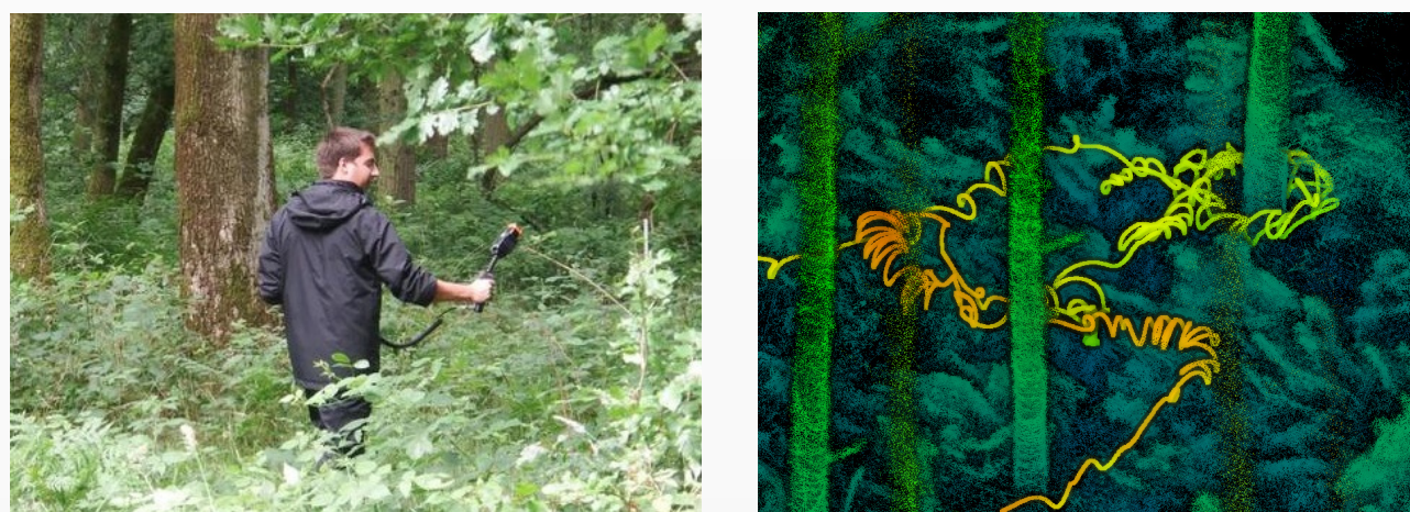
Above-left: a photograph illustrating the author collecting data with a GeoSLAM ZEB-1 handheld laser scanner in one of his forest field plots.
