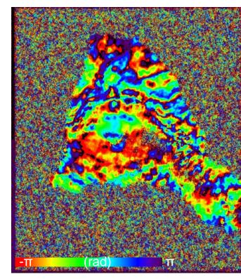
An example of the phase due to the low frequencies of the interferograms 20170923\_20170929 and 20180202\_20180208, after removing the phase correlated with topography from the respective interferograms using Fourier transforms.
