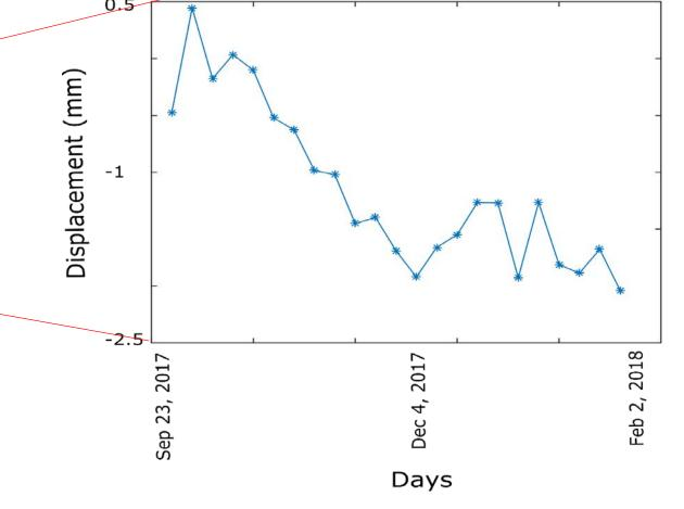
The figure above shows the accumulated deformation using the filtering and the standard PSIG chain. It shows a significant improvement in the spatial coverage of PSs and reduction in phase unwrapping errors. Also an example of the time series of a stable point is shown in the figure.
