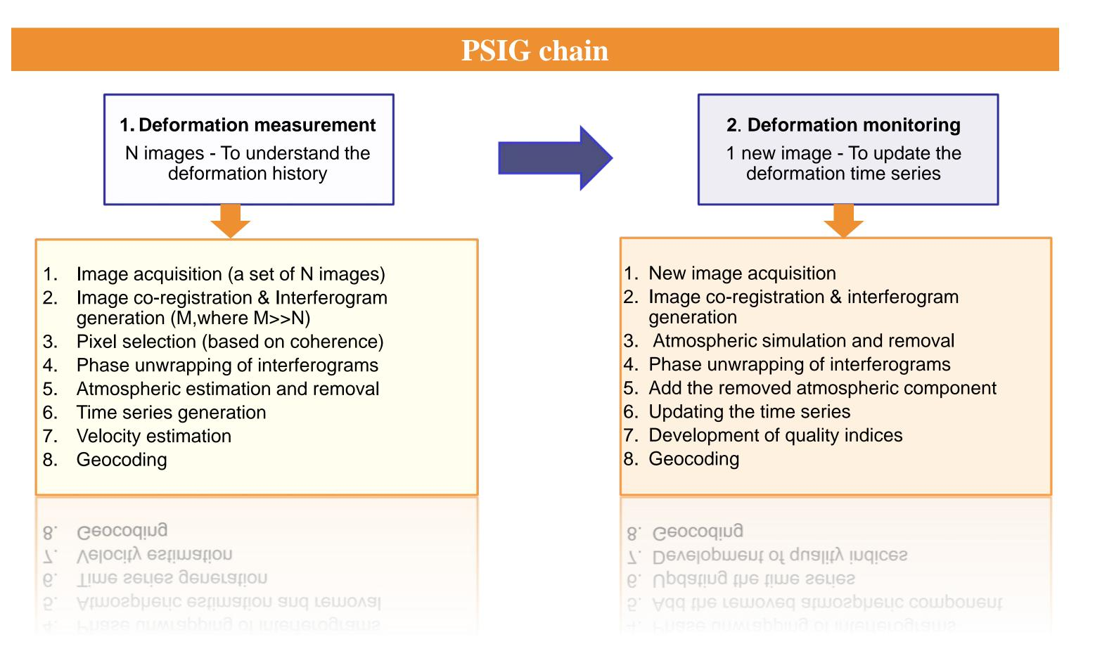
The main objective of the PSI chain was to extend interferometric processing to wider areas using a unique, redundant and connected network of points and any type of interferometric SAR data. The generated maps consist in a set of selected points (Persistent/Dispersed Scatterer (PS/DS)) containing the information of the estimated annual velocity and the accumulated deformation at each image acquisition time.
