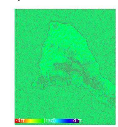
The phase of the residuals after of filtering the low frequency signals is shown in the figure. By preliminary qualitative analysis, it was observed that most of the deformations or movements existing in the given area was retained in the image
