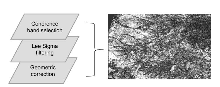
1. Generation and processing of the interferometric C-band coherences as proposed by the ESA.
