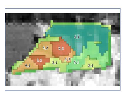
The Tables present the values of the average NDVI delivered on the basis of Landsat 8 satellite data acquired shortly before the harvest, which were calculated within the homogenous polygons, elaborated on the basis of bare soil.
