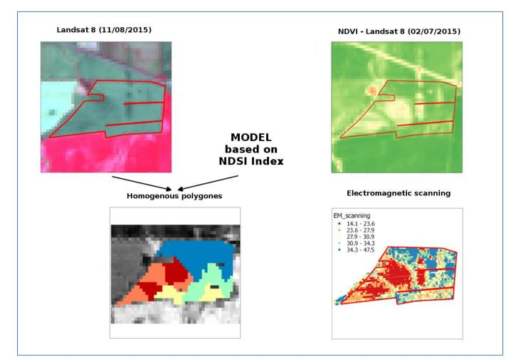
The comparison of homogenous polygons map with the map of NDVI, delivered on the basis of Landsat 8 satellite data, acquired in the end of growing season.
