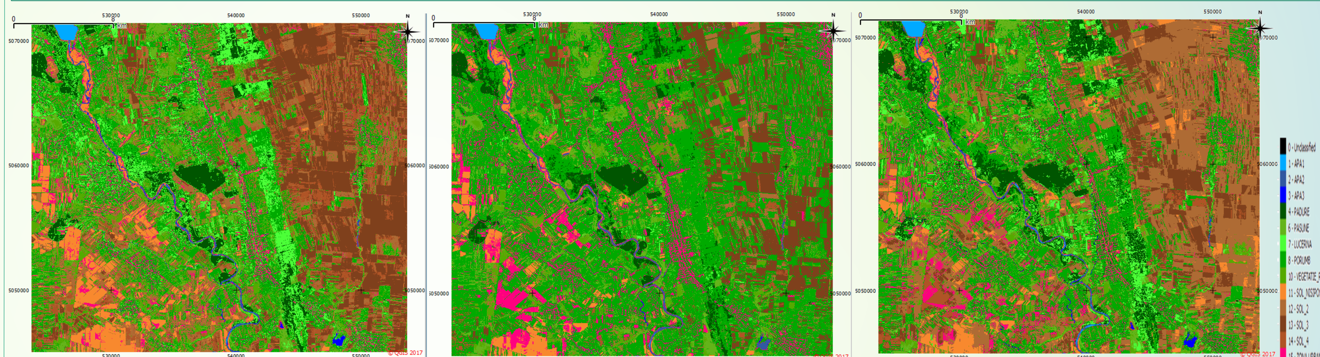
Figure. 4 Supervised classification, based on classes, using a) Spectral Angle Mapping; b) Maximum Likelihood; c) Minimum Distance.
