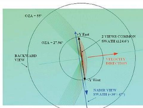
Backward inclined (left) and near nadir (right) views of the scanning mirror geometry
